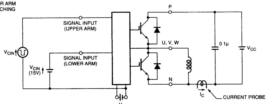
Figure 4 Switching Time Test
