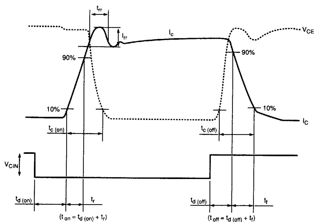
**Figure 5 Switching Test Waveform**
