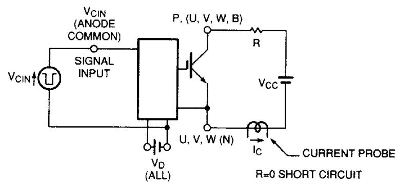
**Figure 7 Over Current and Short Circuit Test**
