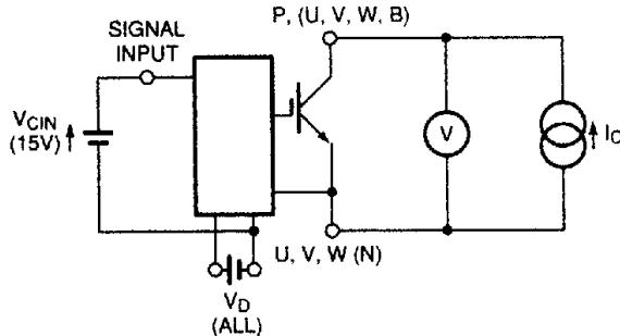
Figure 1  $V_{CES}$  Test
