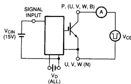
**Figure 6  $I_{CES}$  Test**
