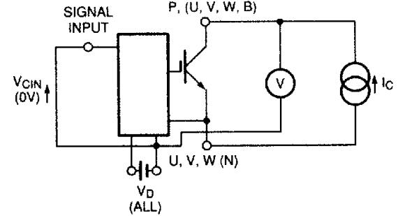
Figure 2  $V_{CE(SAT)}$  Test
