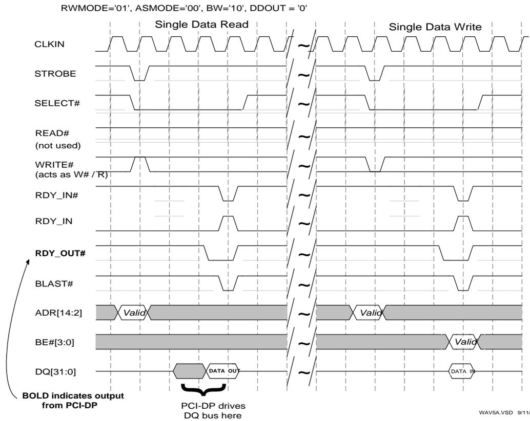
Use RWMODE = '10' or RWMODE = '11' to interface to a processor that has separate active LOW read and write signals. The two modes are identical. Sampling of the READ and WRITE signals is used as the internal address strobe in place of the STROBE signal. This is illustrated in Figure 15.
